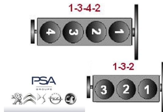
Example of PSA cylinder numbering Beware: First cylinder at gearbox side.
