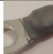
6. Detail of correct insulation.
