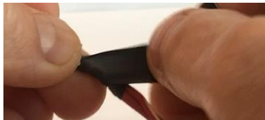
2. Stretch the tape to 3/4 of its original width during application
